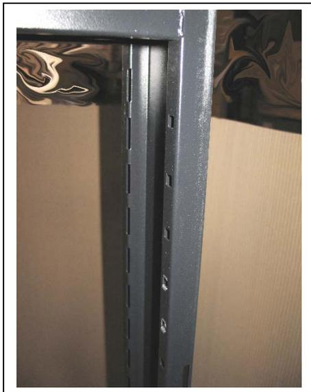
For best fitment use holes 5 & 6 from top and bottom on vertical profiles and holes 22 & 23 on horizontal support bars
