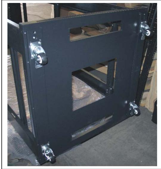
Attach the supplied Cabinet Base to the bottom of the Cabinet frame. Ideally the frame assembly should be parallel to the ground to help make installation of the base easier.
